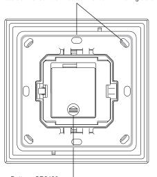
Battery: CR2430 Before the first use, please open the battery cover and remove the protective film
